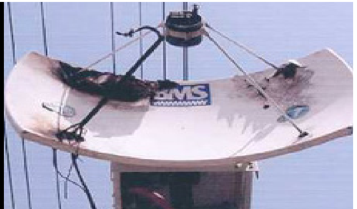
The actual antenna and transmission dish that showed visual evidence of the wire contact location and resultant burning.
