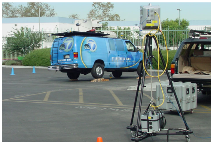
Laser Scanner with Exemplar Van
