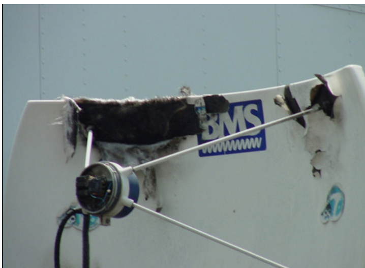
Photo of Burned Antenna
