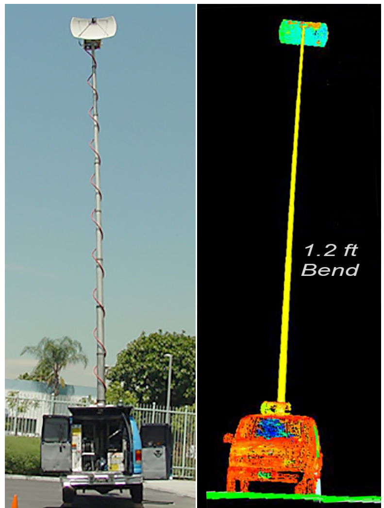
Photo with Elevated Wheels and Laser Scan Showing Antenna Bend
